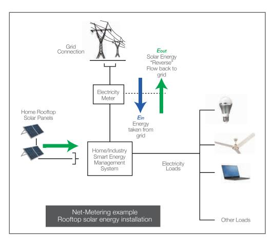
The diagram above<sup>44</sup> helps illustrate the concepts of net metering, and associated concepts of feed-in tariff and reverse metering.
