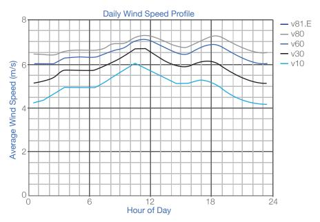
Figure 11: Diurnal Wind Speed profile for Baburband Mast.
